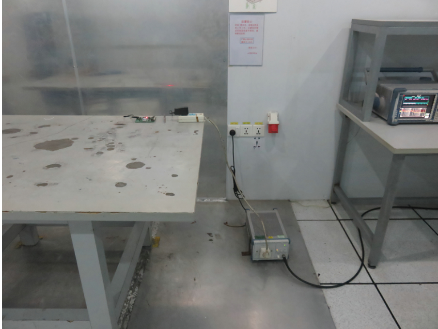
Photo of Conducted Emission Test
