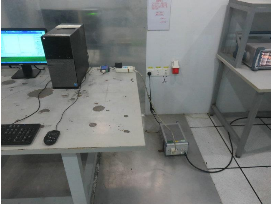
Photograph – Conducted Emission Test Setup
