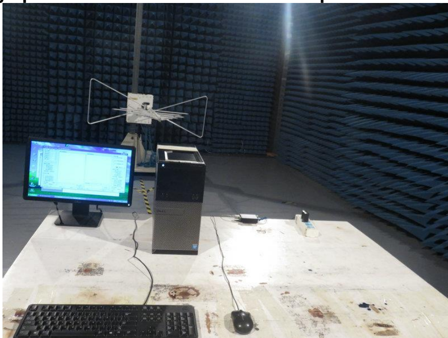
Photograph – Radiated Emission Test Setup
