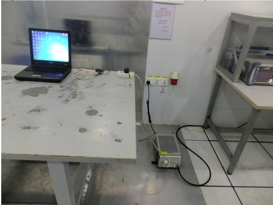
Photograph – Conducted Emission Test Setup
