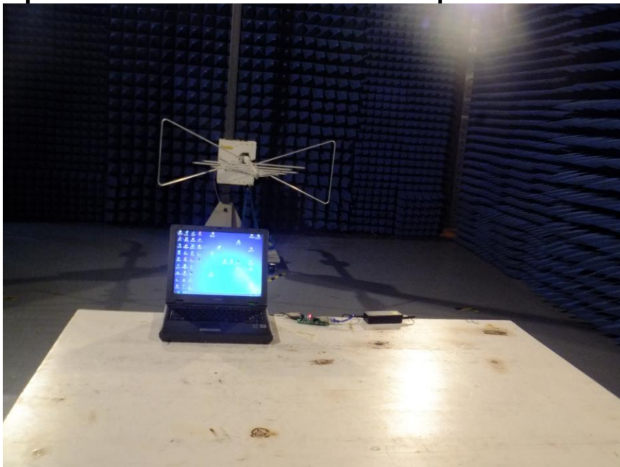
Photograph – Radiated Emission Test Setup
