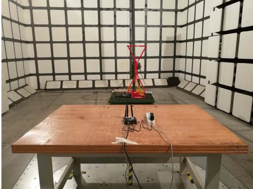
Radiated Emissions View (Below 1 GHz)
