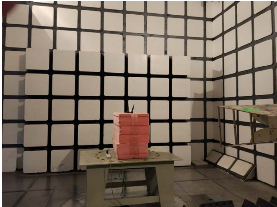
Radiated Emissions View (Above 1 GHz)
