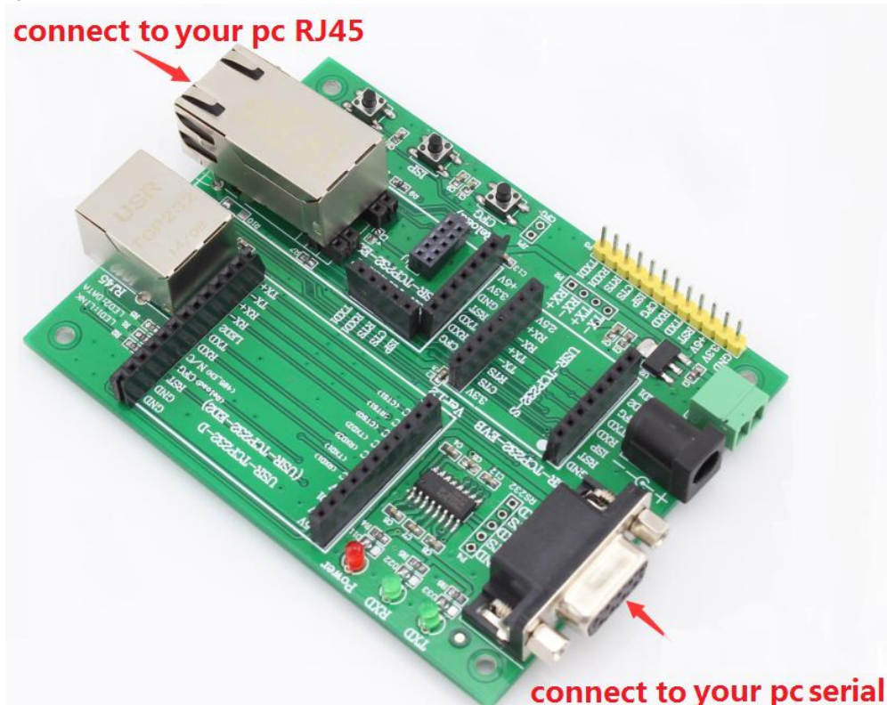
Diagram 2-1 USR-K1 Connection diagram
