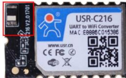
Figure 8 USR-C216a antenna part
