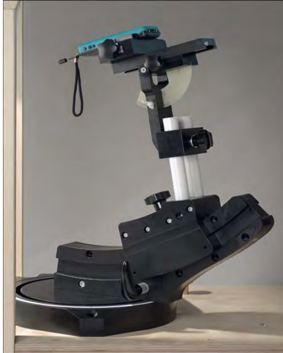
F-2. Device Holder for Transmitters
