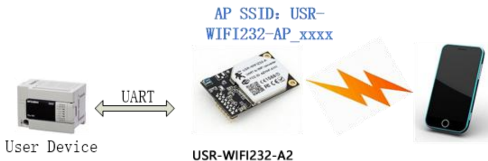
Figure 47 Wireless Control Application
