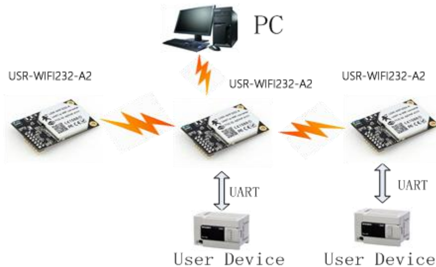
Figure 17 USR-WIFI232-A2 STA Network Structure
