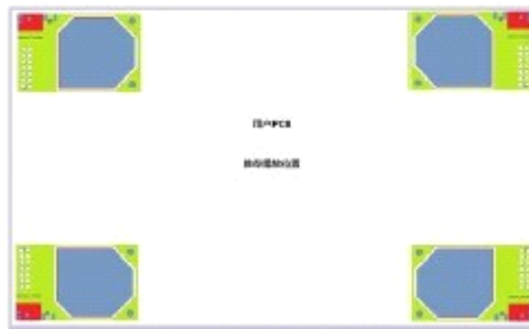
Figure 12 Suggested Module Placement Region
