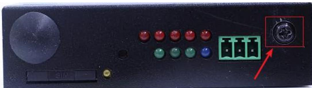
Grounding screw installation:
