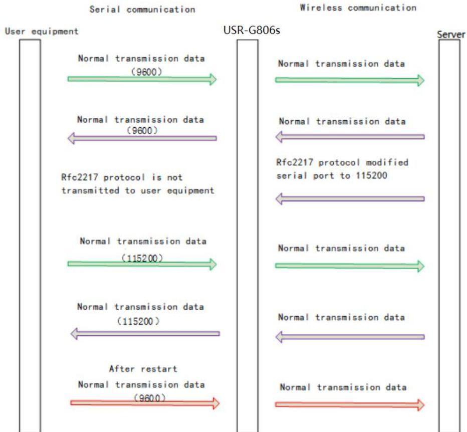
This function is similar to RFC2217, when we send the specific protocol data from the network side, can change the serial parameters in real time. Parameters take effect immediately, but it will be restored to the original after restarting.
