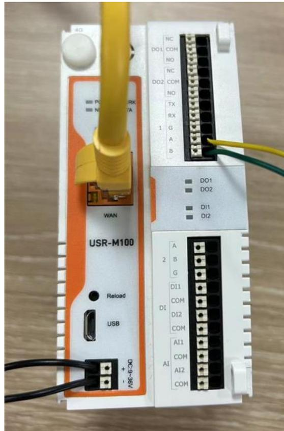
Fig. 10 Hardware connection
