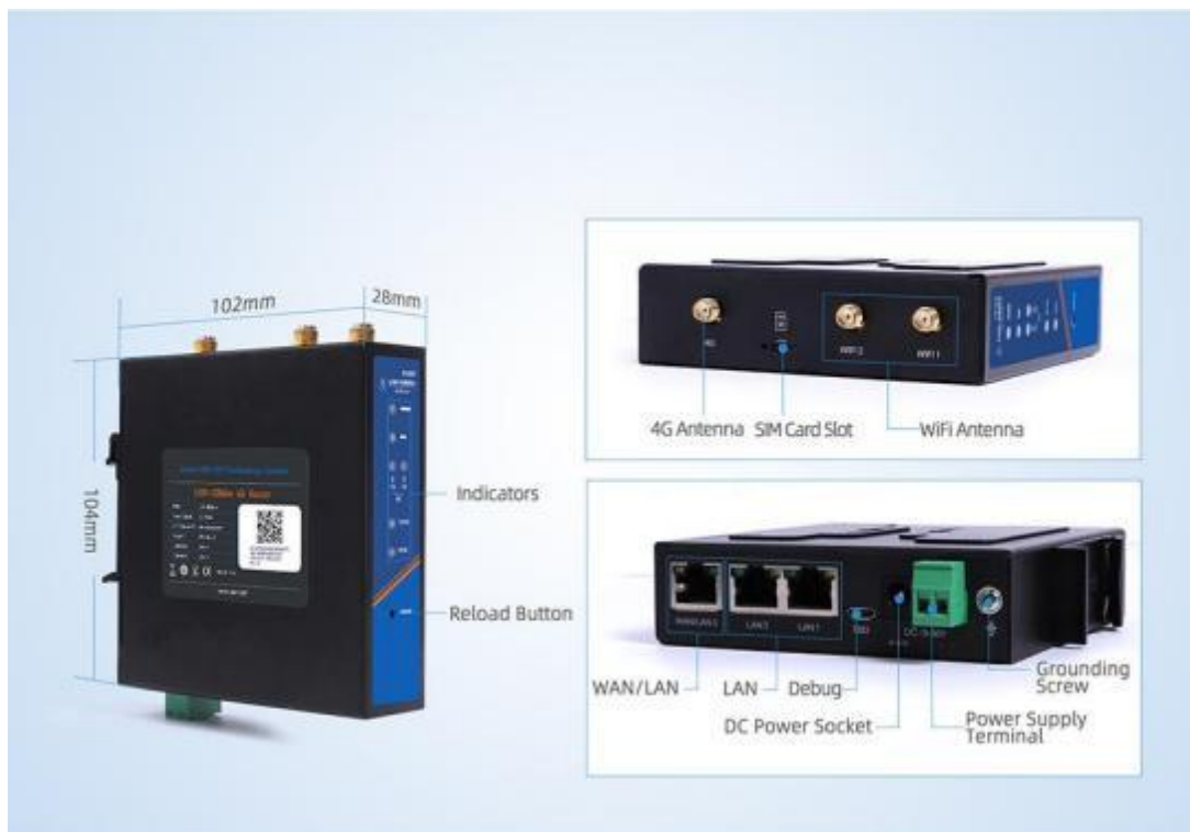
Fig. 1 Hardware interfaces
