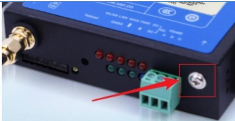
Grounding screw installation:
