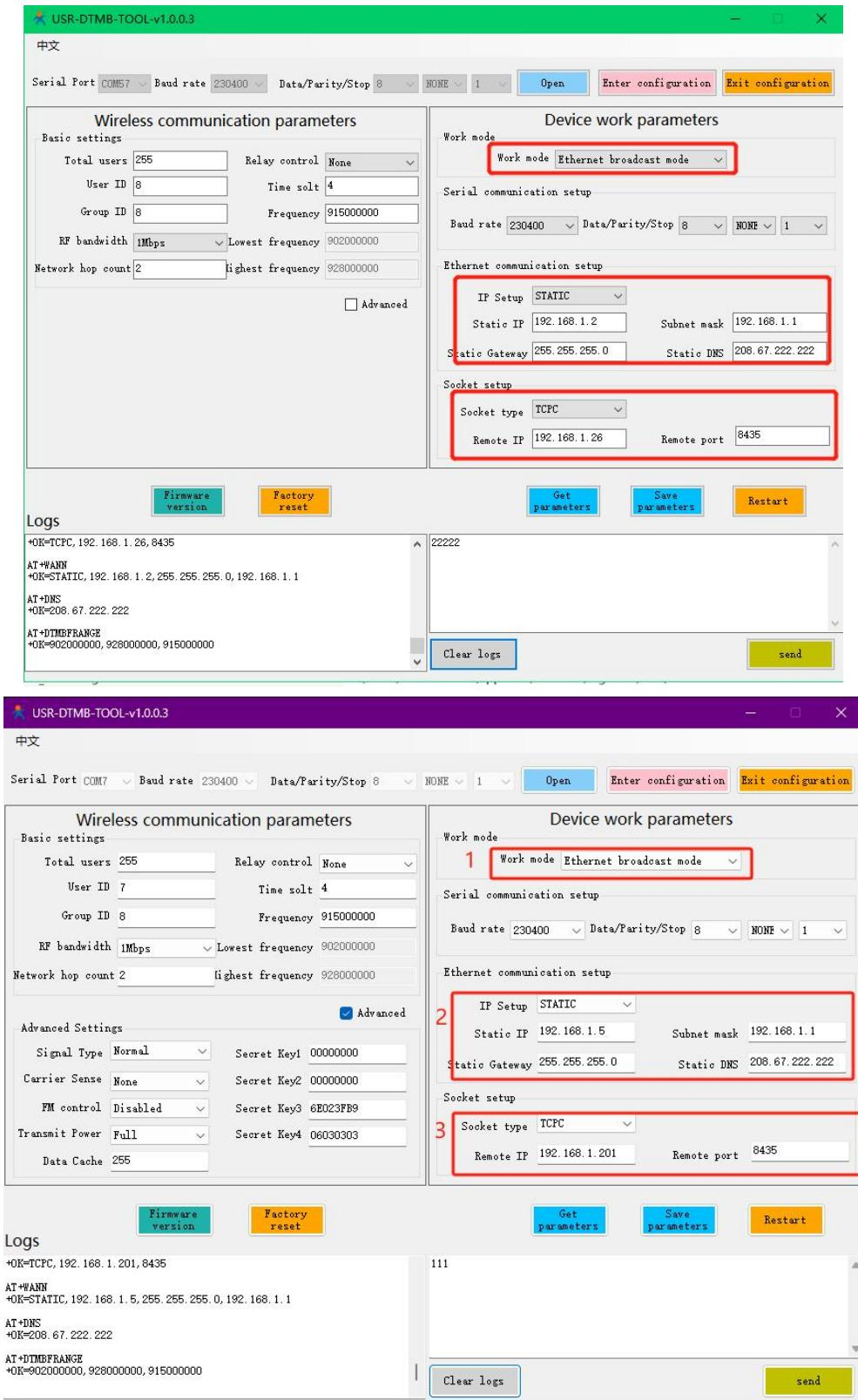
(2)Set the static IP address of the computer, as shown below.
