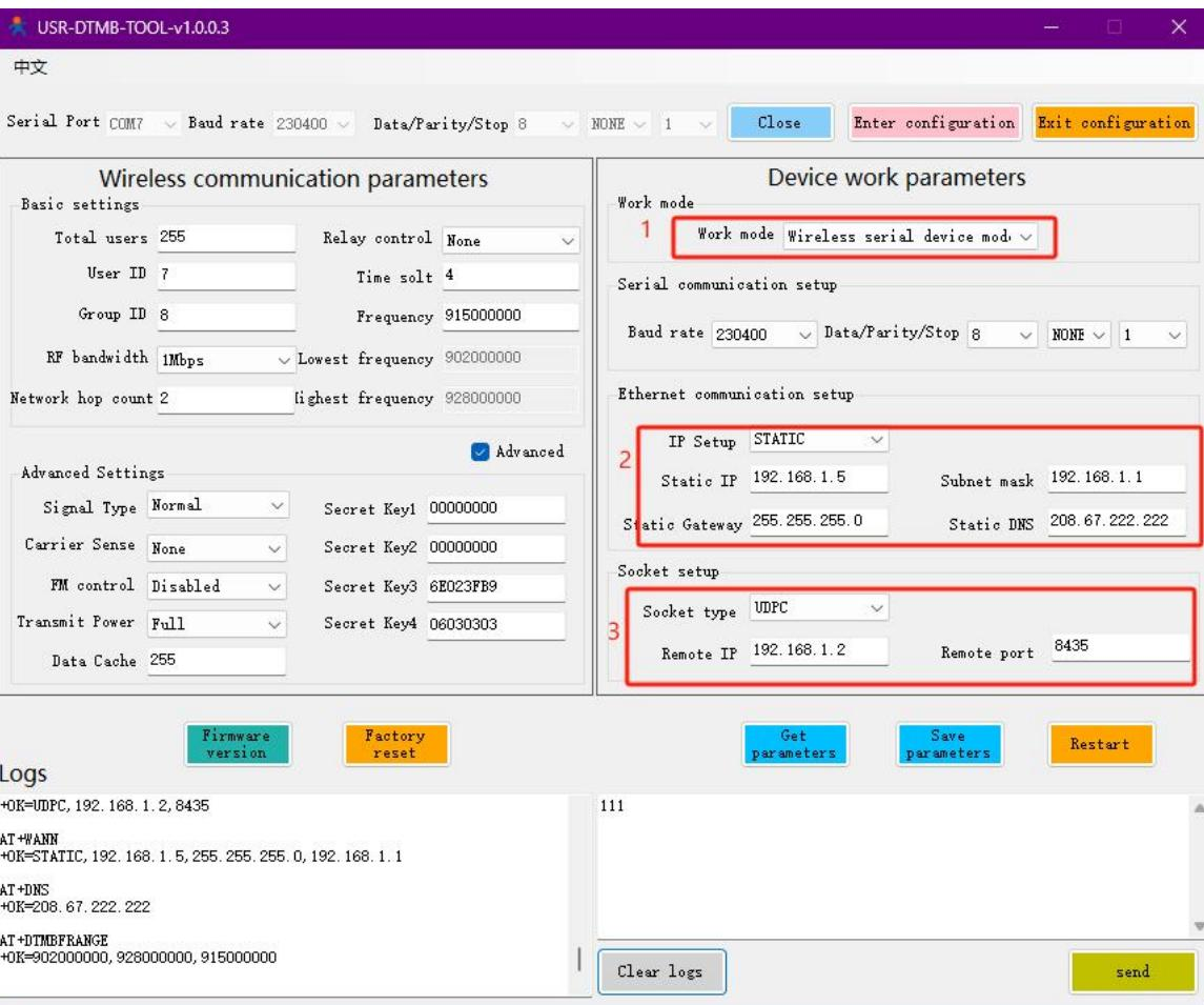
(2) Restart after setting and send data to serial port respectively
