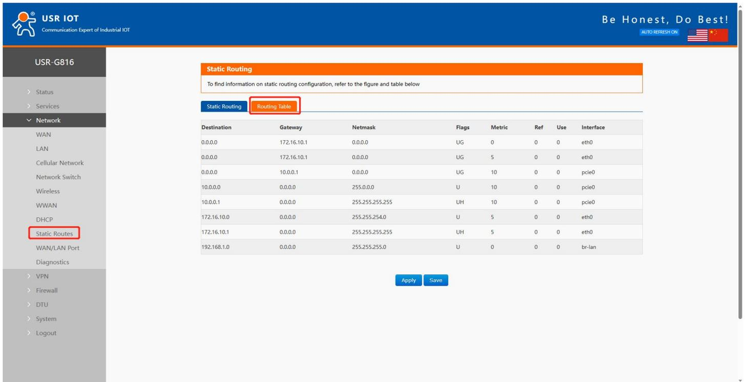
Figure 30. Routing table checking
