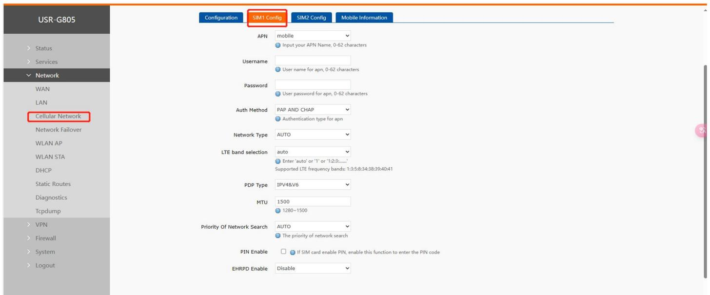
Figure 20. SIM card configuration
