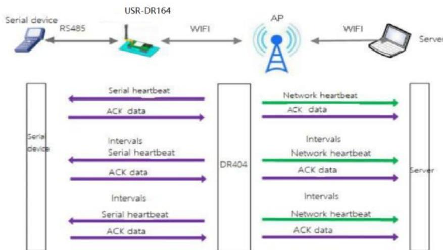
The main purpose of sending to the network is to maintain a connection with the server, and at the same time let the server that is idle for a long time (do not send data to the server for a long time) to detect whether the current connection status is valid.
