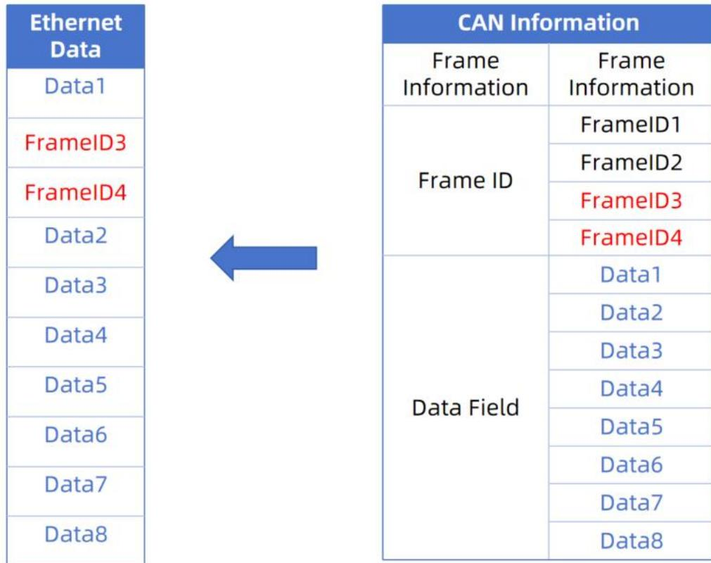
**38.Transparent tape ID transmission--CAN to serial frame**
