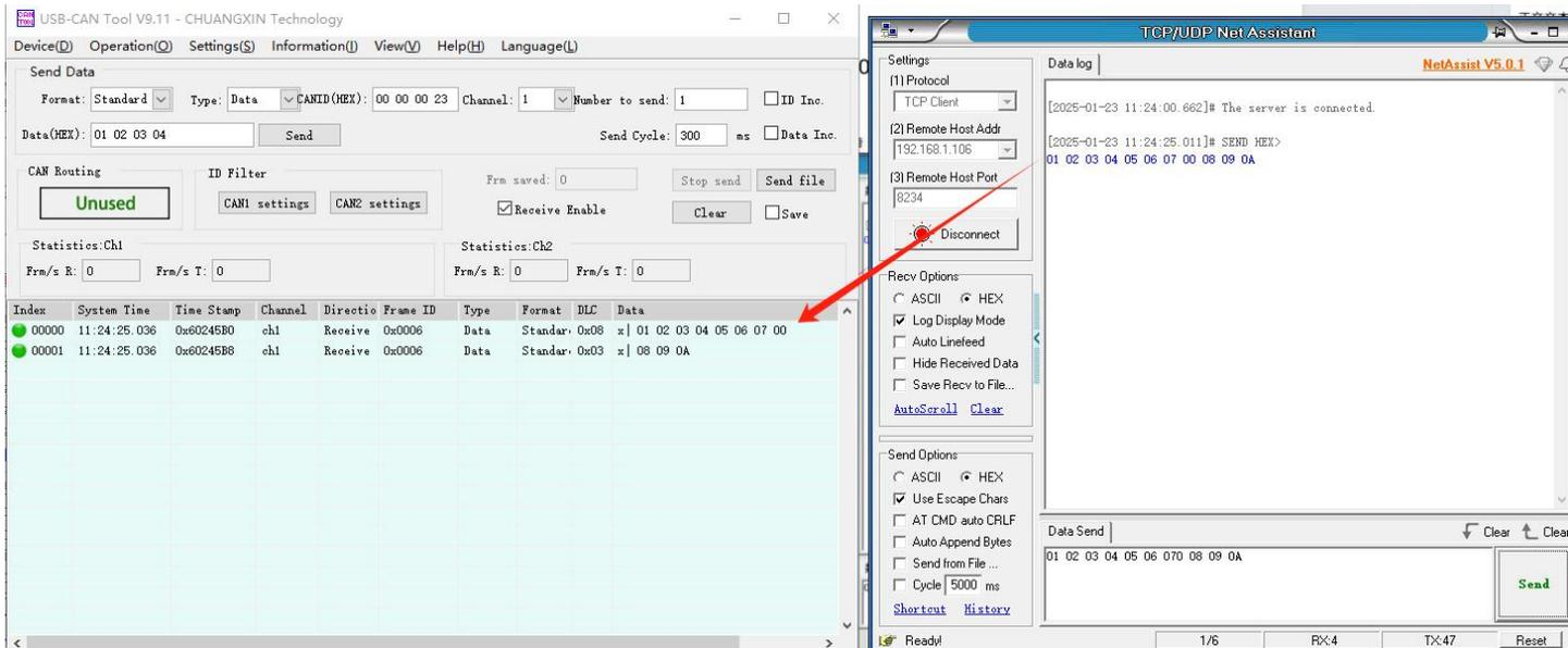
**33.Transparent Transmission--Ethernet Data to CAN Transmission Example**
