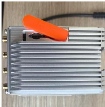
4、 Attach 4G/Wi-Fi antennas and GPS antenna (GL version only).
