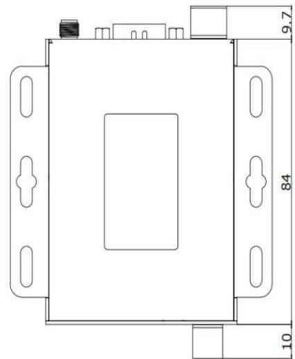
Sheet metal shell, fixing holes on both sides;
