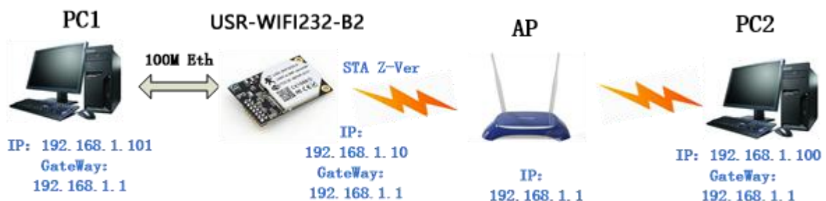
Figure 21 USR-WIFI232-B2 Ethernet Interface Networking (As STA, Z-Ver)
