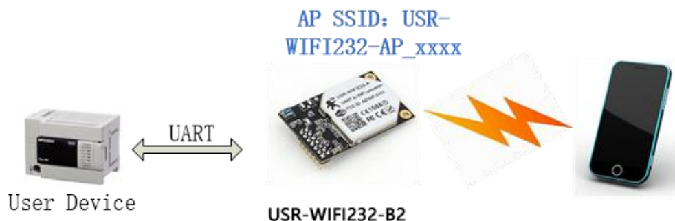
Figure 47 Wireless Control Application
