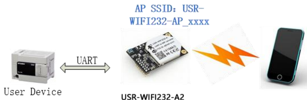
Figure 47 Wireless Control Application
