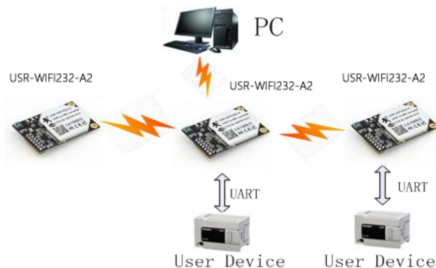
Figure 17 USR-WIFI232-A2 STA Network Structure
