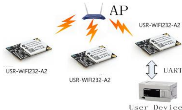
Figure 16 USR-WIFI232-A2 Basic Wireless Network Structure
