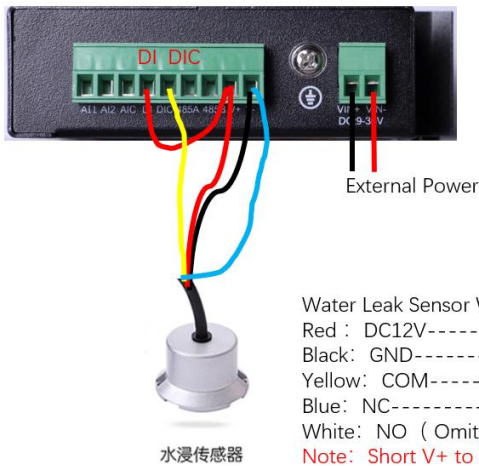
Wiring Diagram Type 1: Passive Dry Contact Digital Input
